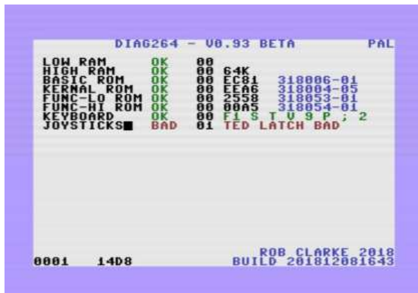
Screenshot 6 - Failed TED Latch
